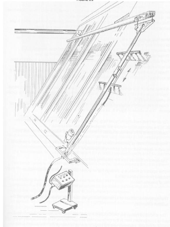
Fig. 8 Automated Cleaning Machine
