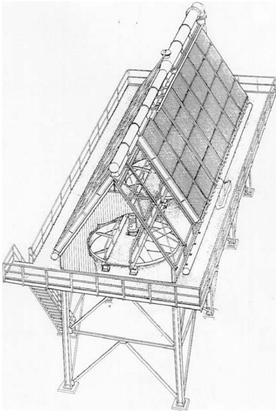
**Fig 1. General View of Air-cooled Condenser**
