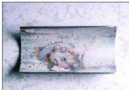
Figure 2. Pitting under scale in stainless steel tube.
