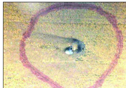
Figure 3. Erosion-corrosion around deposits.
