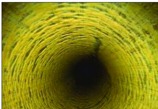
Figure 8. Stainless steel condenser tube with calcium carbonate scale.
